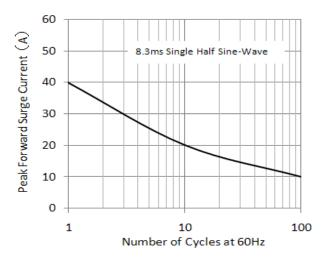
Figure 2.Maximum Non-Repetitive Peak Forward Surge Current
