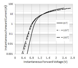
Figure 3. Typical Forward Characteristics
