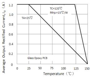
Figure 1.Output Rectifier Current Derating Curve
