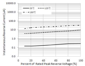
Figure 4. Typical Reverse Characteristics
